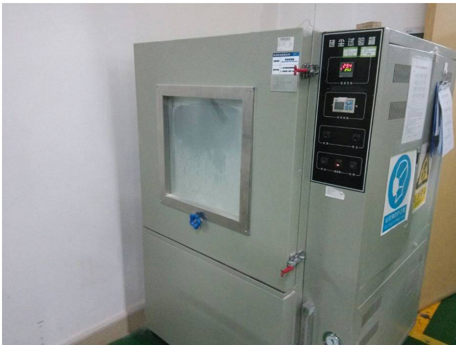
Testing of IP6X
