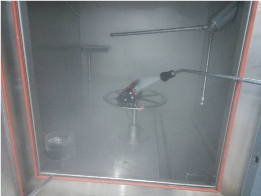
Testing of IPX9K (60 degrees)
