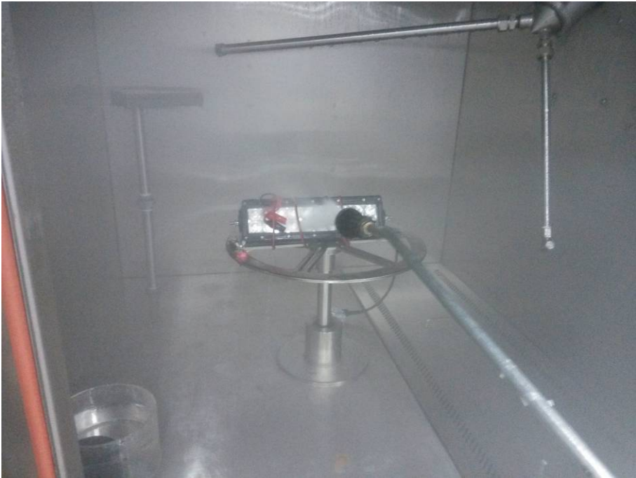
Testing of IPX9K (0 degrees)
