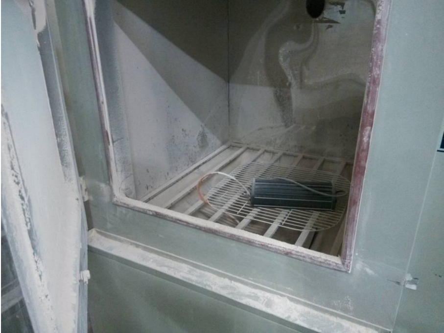
After the test of IP6X
