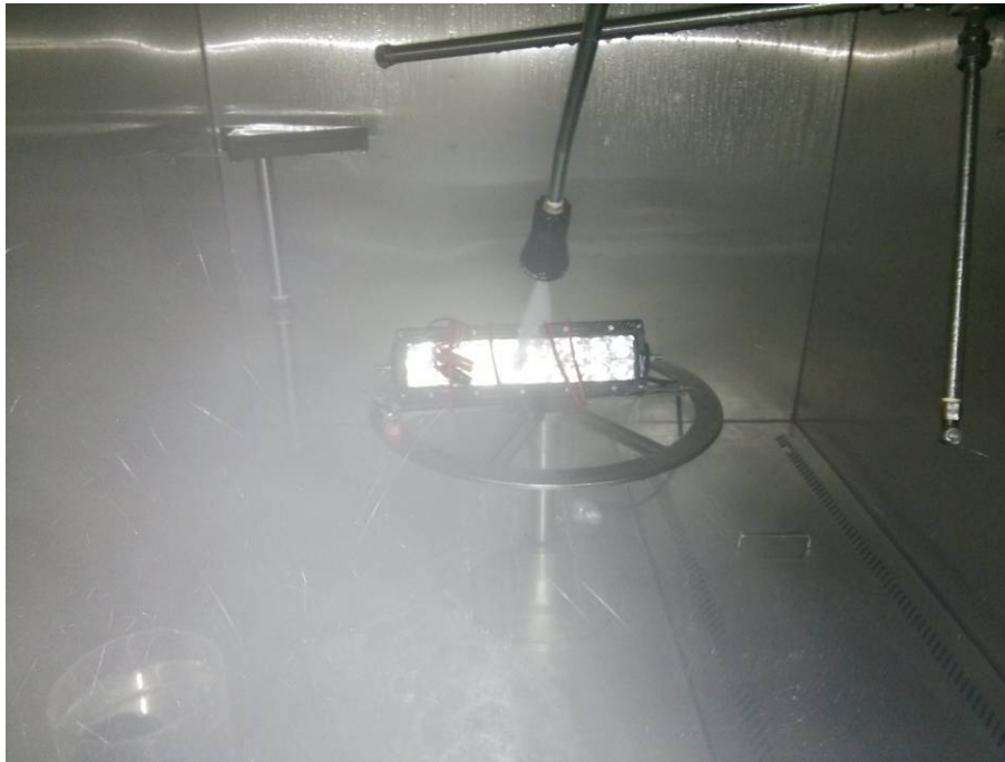
Testing of IPX9K (90 degrees)
