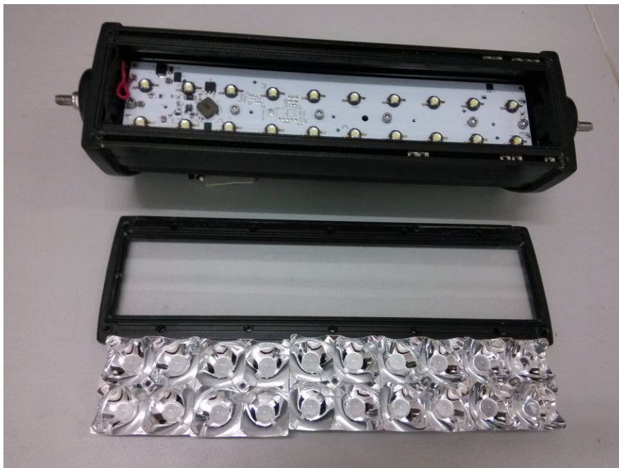
Result for the test of IPX9K
